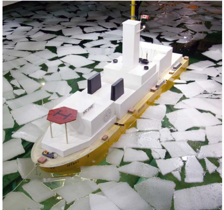
A model scale drilling platform undergoes dynamic positioning tests in ice at the world's longest ice tank, located at the NRC Institute for Ocean Technology.
